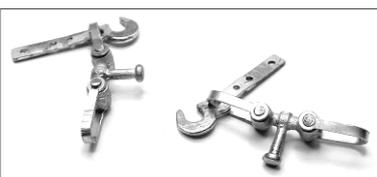
Pass the coupling hook through the slot and retain it with a length of spring wire. Polish the centre of this wire with emery cloth first so that you can solder it to the coupling hook shank once you are happy that the buffers spring freely.
