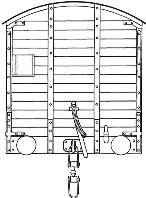
LNER Livery. Bodywork including solebars and headstocks, Red Oxide. Roof, white later grey. Running gear and buffers, black. Lettering, white, pre 1936 as drawing. Post 1936 the 'NE' was reduced to 4", placed over '12T' in 3" which in turn was above the running number in 4". All to the bottom L/H corner with 3" spaces between lines.
