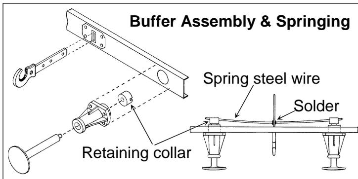
Cosmetic screw coupling. Solder both halves of each hook together and if necessary round the slot so that the link will swing freely and then using round-nosed pliers form the four links into U shapes. Dress the tops of two links with a file so that they will pivot freely in the slot in the hooks. Thread one of these links through the hook and spring the ends over the pegs on the cast centre.
